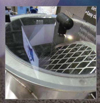
Angel Hair can wrap around augers, cause material to bridge hoppers, and contaminate the system. An Advanced Blending Solutions' Angel Hair Trap can remove these stringers before they become a problem. Angel Hair Traps can also be used as a tool to pinpoint where Angel Hair is being created. Install several or move them around a resin system to find problem areas. Angel Hair Traps are designed for use in vacuum lines only.
